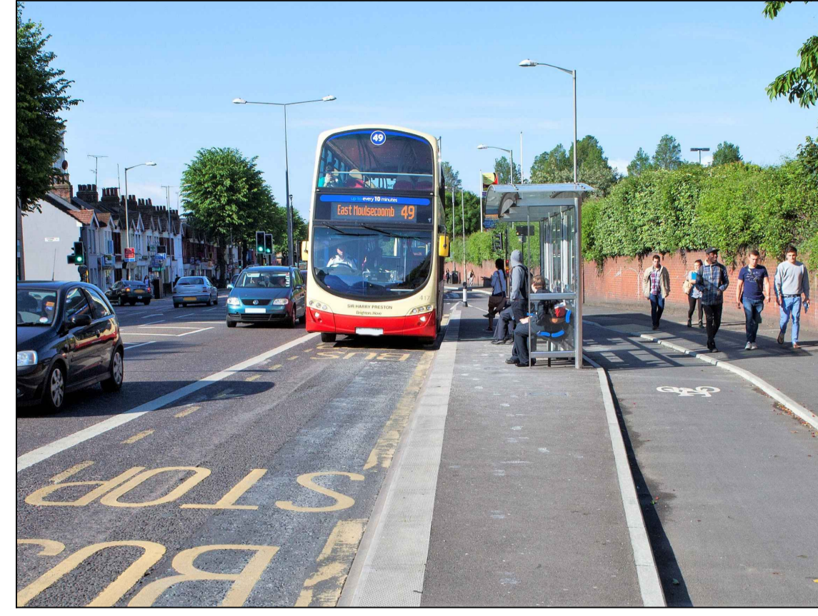
Image 2 - Example of floating bus stop
